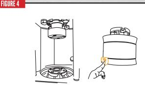
Remove the old ram, clean the bore of the barrel and spread the grease onto the new ram and bore.
