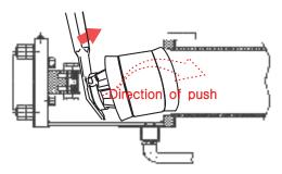
Put the bottom side of the ram into the concrete cyl. and push it DOWN  $\Rightarrow$  UP by using the lever.
